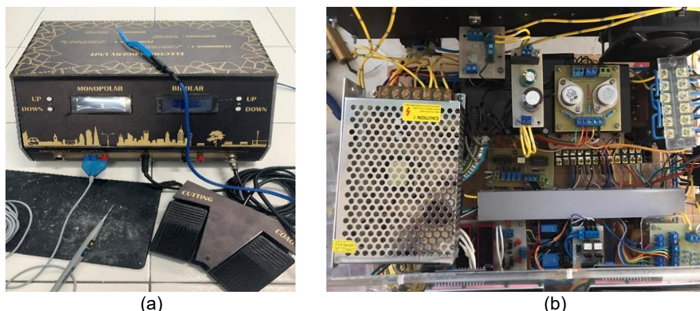
FIGURE 1. (a) Electro-surgery unit module hardware form and circuit. (b) Electro-surgery design consists of analog and digital circuits. Analog circuit is in the form of pulse adjustment button, buzzer, power adjustment, pulse adjustment, oscillator, driver, and inverter. The digital circuit is a microcontroller system controller and an LCD display. The design of the device was made in such a way to adjust the needs and safety of the circuit. The footswitch port, plate, and active electrode were also placed in front of the device to facilitate installation and user movement.
