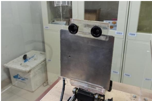
FIGURE 6. The Simple Collector Made by Flat Plate
