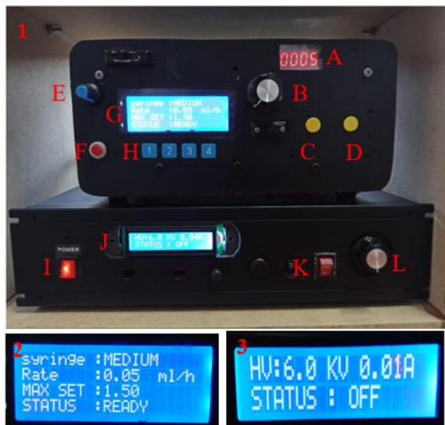
FIGURE 9. Syringe Pump and High Voltage Power Supply Setting Management
