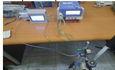
FIGURE 1. The installation of data collection from the oxygen cylinder so that it can be read by the oxygen flow analyzer module, consisting of the oxygen cylinder, the oxygen analyzer module, and the standard gas flow analyzer (IMTMedical) as the comparison device
