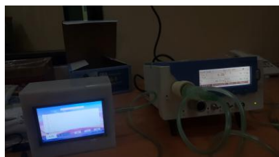
FIGURE 4. Data retrieval by stringing a series between the oxygen cylinder, module, and oxygen flow analyzer
