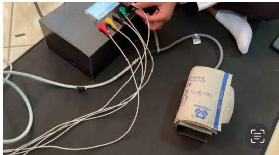
FIGURE 4. Installation of ecg and NIBP cables to the monitor module and patient
