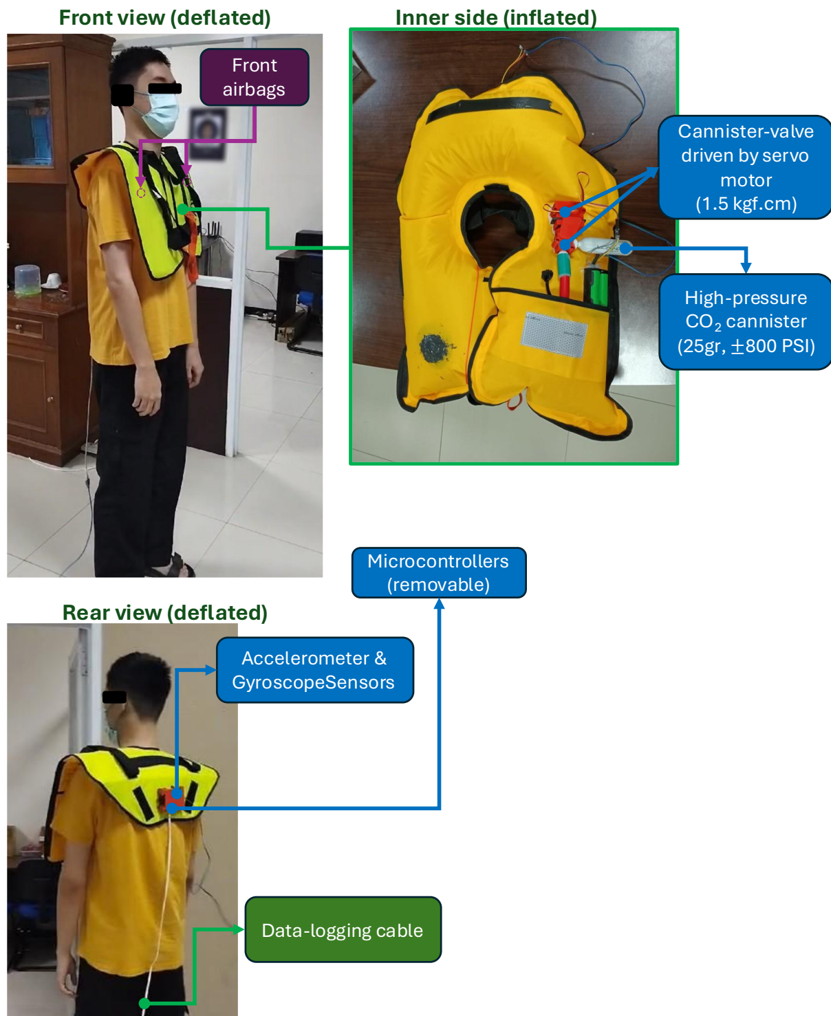
Fig. 1. The proposed lightweight safety vest with inflatable airbag.
